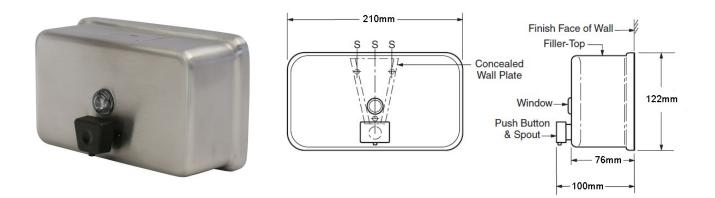
Model WA0345 is our wall mounted stainless steel horizontal liquid soap dispenser. All surfaces polished to a satin finish. Supplied with concealed fixings and holds 1.2 litres of liquid soap. The soap reservoir is provided with a hinged lockable cap to resist vandalism.
